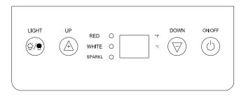
You can select temperature display setting from Fahrenheit to Celsius degree by holding down UP and DOWN buttons at the same time for three seconds. Fahrenheit or Celsius degrees indicator will appear in blue color in the temperature display window.
